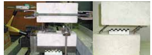
Stitch-Tie testing for shelf angle support
