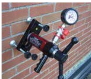
Mortar Joint Performance Test
